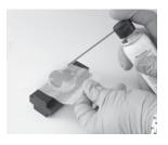
Apply a couple drops of lens cleaning fluid to the lens paper (far side of the lens).
